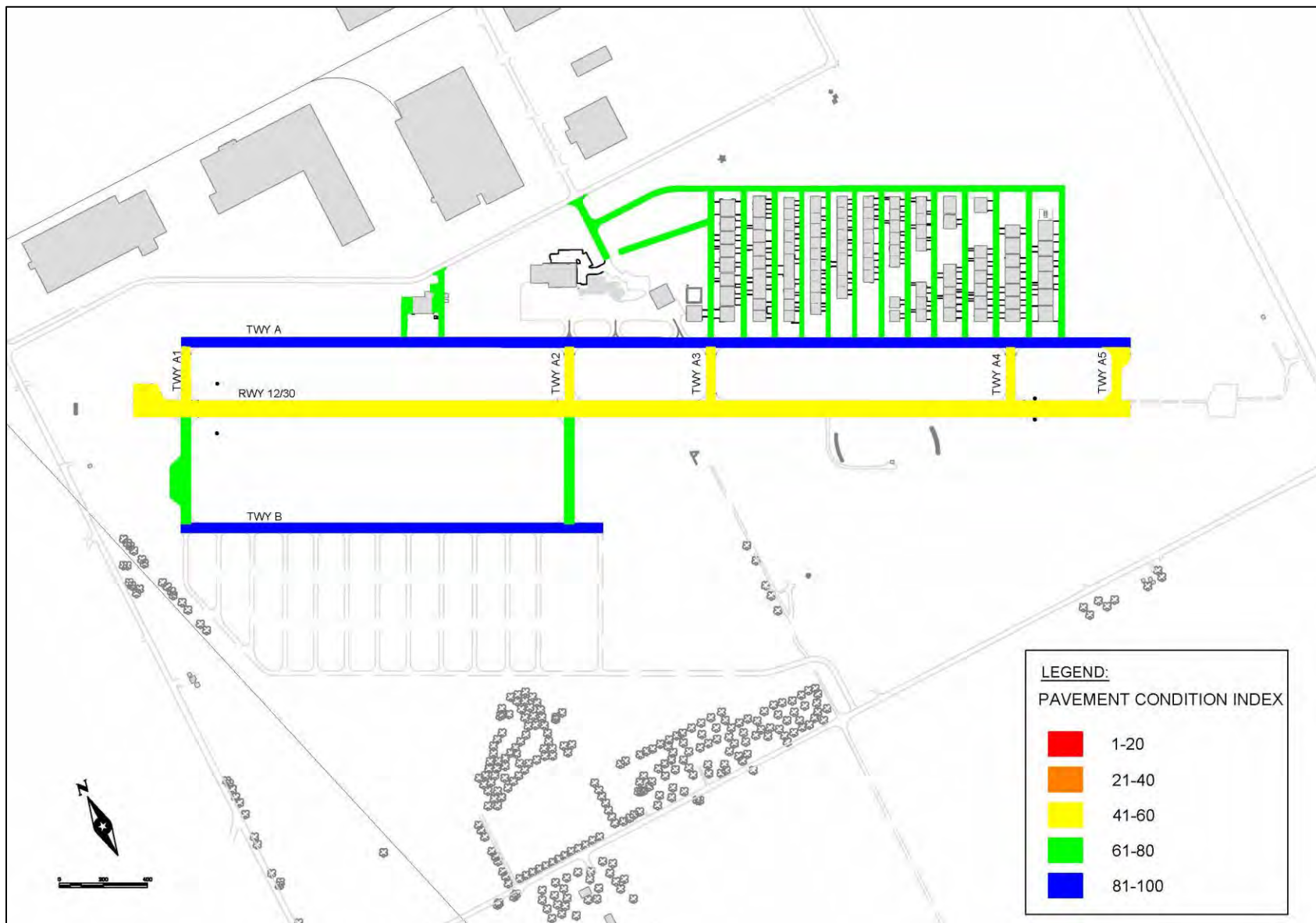
Figure 2-2: Airlake Airport Pavement Condition Index (2016 PCI)
