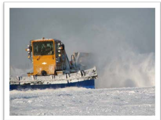
MAC High Speed Plow Removing Snow from the Runways
