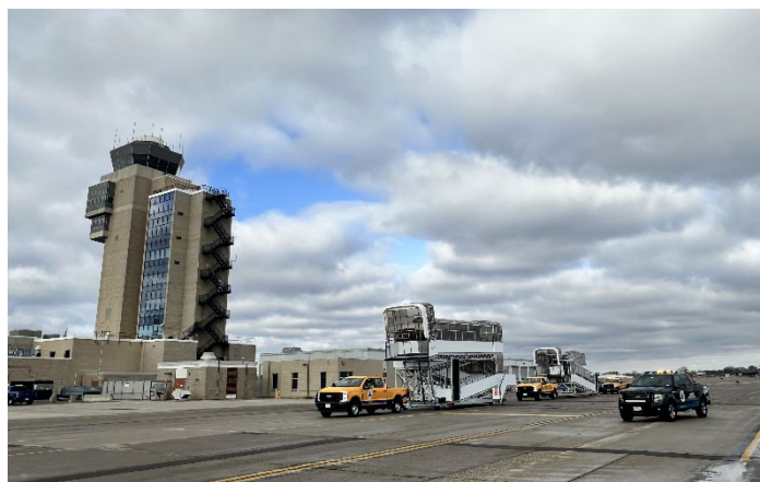
Step-Free Aviramps, a More Accessible Alternative to Traditional Airstairs, are Used for Emergencies
