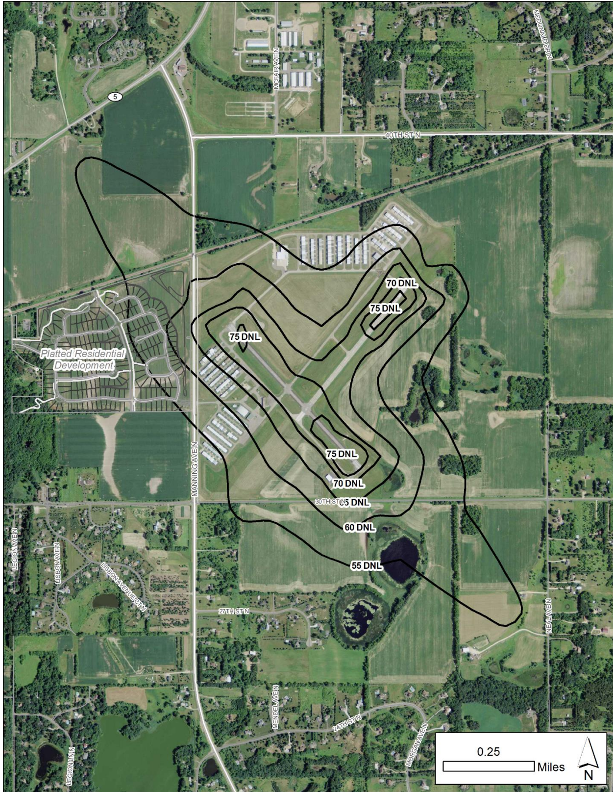
Figure 6-3: Baseline Condition Noise Contours
