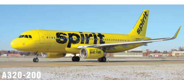
**Number of seats: 178** Seating: 3-3 Speed/mph: 530 Range/nautical miles: 3300 Wing span: 117 feet 5 inches Overall length: 123 feet 3 inches Cabin length: 90 feet 3 inches Fuselage width: 13 feet
