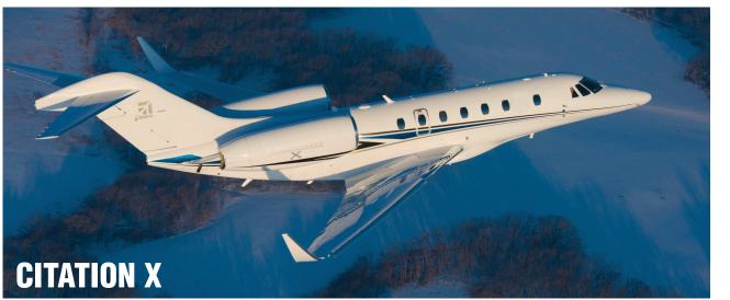
**Number of seats:** 11 to 14 **Speed/mph:** 528 Range/nautical miles: 3300 Wing span: 63 feet 11 inches
