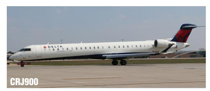
**Number of seats:** 76 Seating: 2-2 Speed/mph: 544 Range/nautical miles: 1732 Wing span: 81 feet 7 inches Overall length: 118 feet 11 inches Cabin length: 69 feet 5 inches Fuselage width: 8 feet 10 inches
