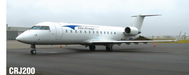
**Number of seats: 50** Speed/mph: 534 Range/nautical miles: 1645 Wing span: 69 feet 8 inches Overall length: 87 feet 10 inches Cabin length: 40 feet 6 inches Fuselage width: 8 feet 10 inches
