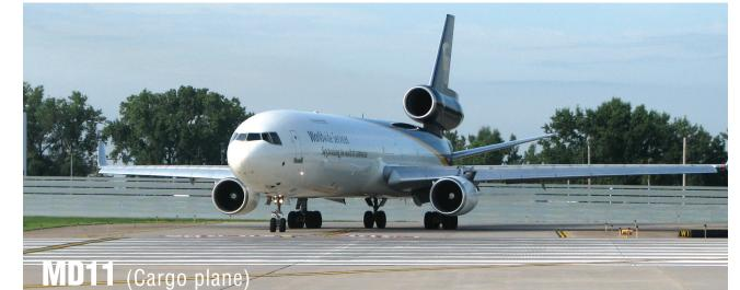
Speed/mph: 544 Range/nautical miles: 7630 Wing Span: 170 feet 6 inches Range/nautical miles: 6920 to 7300
