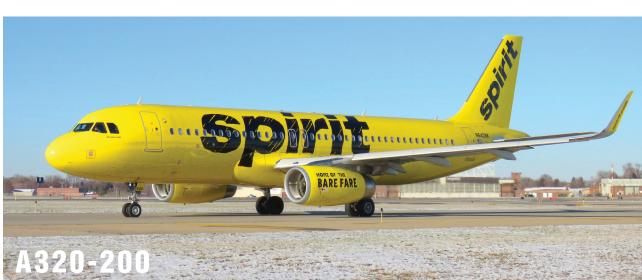
**Number of seats: 178** Seating: 3-3 Speed/mph: 530 Range/nautical miles: 3300 Wing span: 117 feet 5 inches Overall length: 123 feet 3 inches Cabin length: 90 feet 3 inches Fuselage width: 13 feet
