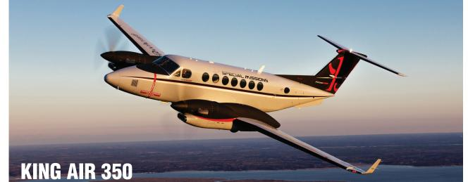
Number of seats: 9 to 11 Speed/mph: 303 Range/nautical miles: 947 Wing span: 57 feet 11 inches
