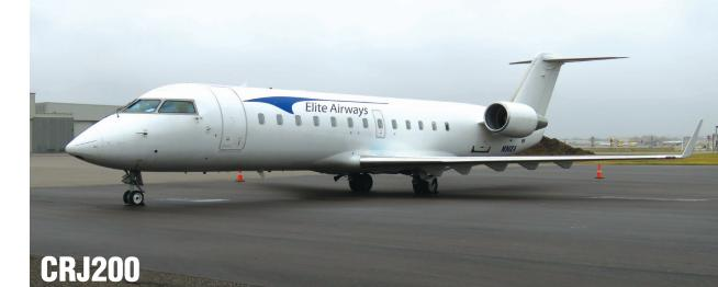
**Number of seats: 50** Speed/mph: 534 Range/nautical miles: 1645 Wing span: 69 feet 8 inches Overall length: 87 feet 10 inches Cabin length: 40 feet 6 inches Fuselage width: 8 feet 10 inches
