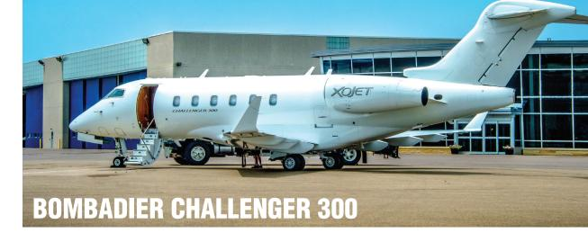
Number of seats: 9 Speed/mph: 554 Range/nautical miles: 3100 Wing span: 63 feet 10 inches
