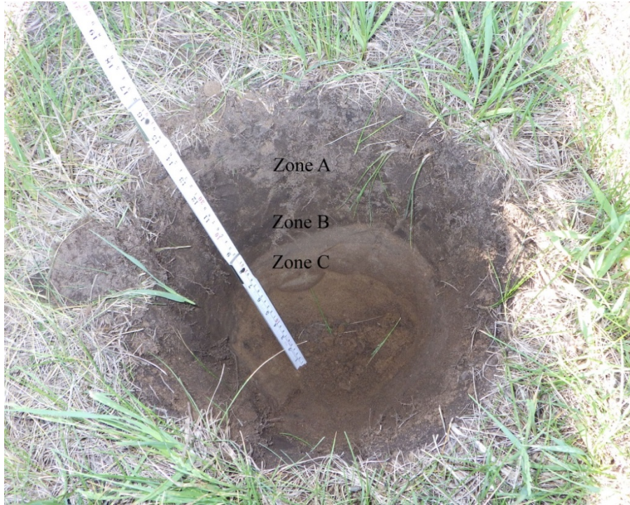
Figure 15. Shovel test at GPS waypoint A002 (Figure 11) in the northwest runway/taxiway reconfiguration, typical for this area of the project. Note the sharp boundary between upper Zones A (10YR 3/2) and B (10YR 2/2), disturbed, and Zone C (10YR 3/6). This particular hole contains a band of black fill (Zone B) under the dark greyish brown topsoil (Zone A).
