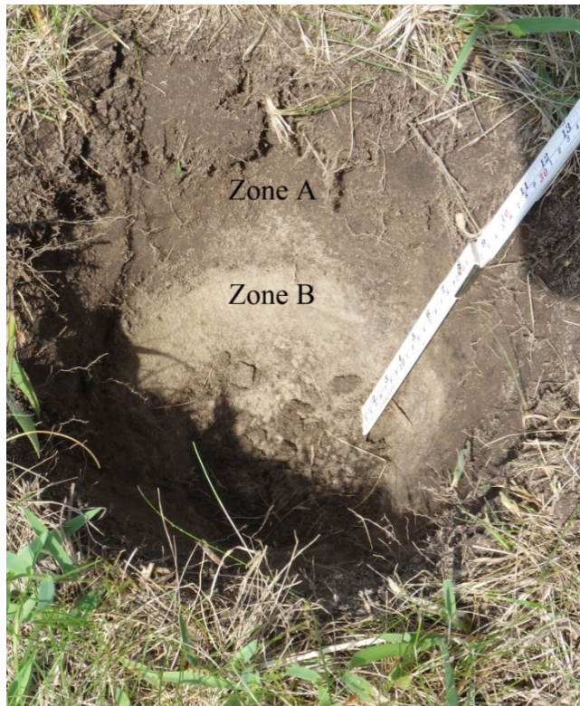
Figure 21. Shovel test at waypoint A014 (Figure 12), illustrative of the hydric soils, seen here in the grey Zone B (10YR 5/1), in the southeast runway/taxiway reconfiguration.
