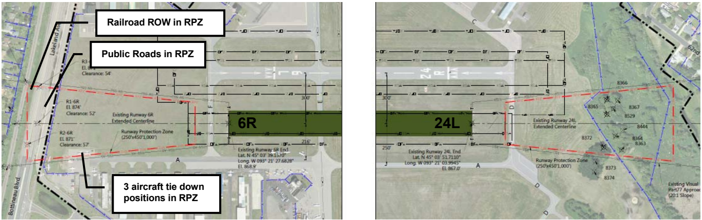
FIGURE 6: RUNWAY 6R-24L EXISTING RUNWAY PROTECTION ZONES
