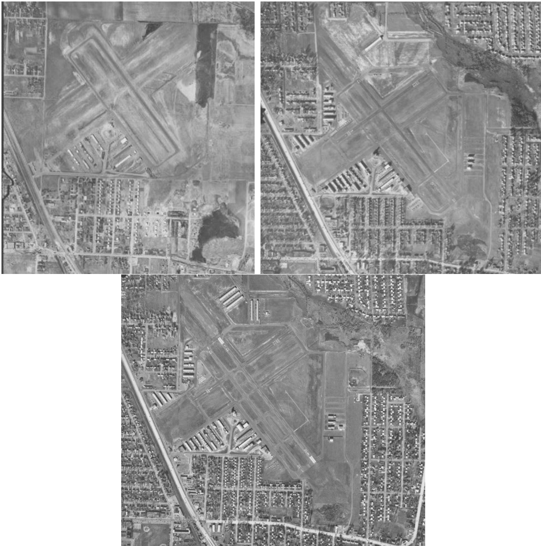
Figures 40 through 42. 1956 (top left), 1967 (top right), and 1971 (bottom) aerial photographs of Crystal Airport. Note the extension of runways (two of which are paved by 1967) and development of airport land. By 1967, Hangar Areas 1 and 2 were developed and the development of Hangar Areas 3 and 4 was just beginning. By 1971, the current runway configuration of three paved and one turf runway is in place. 68
