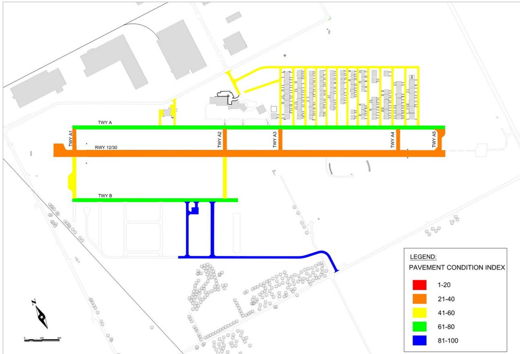
Figure 1-2: 2026 Pavement Condition Index Ratings
