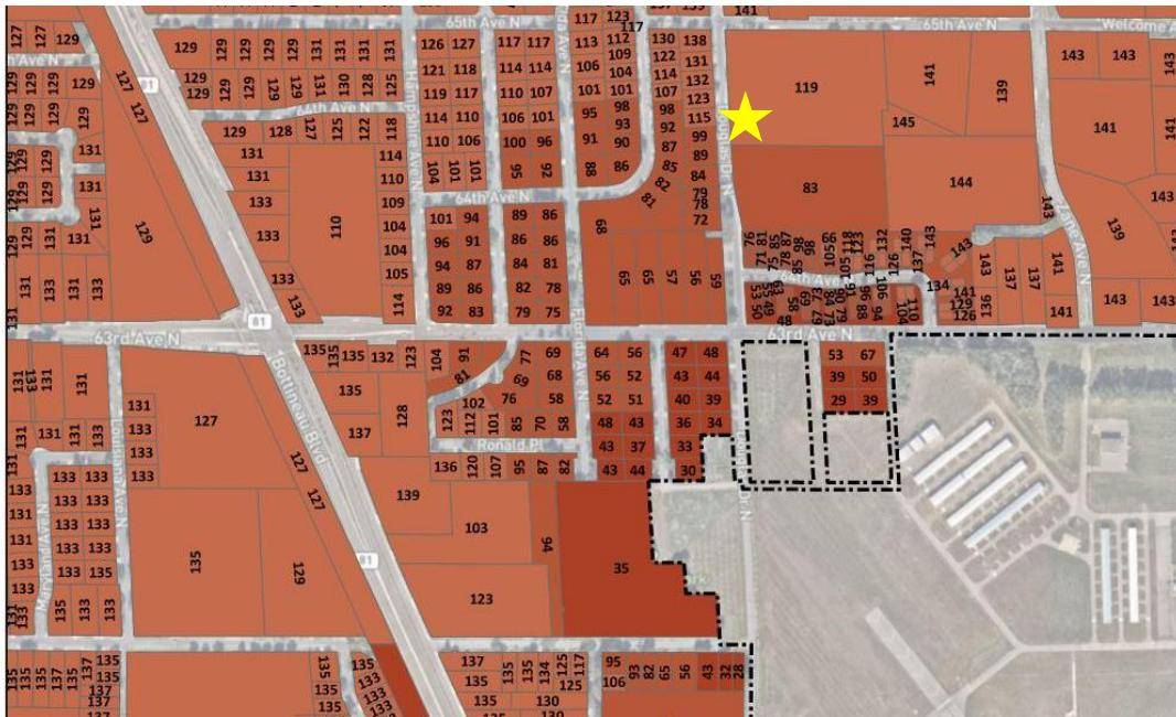
The Maximum Construction Height Without Permit for this parcel is 119 feet AGL (from grid map MCH-C3). The Airspace Zone height at this location is approximately 1010 feet MSL (from grid map A-C3).
