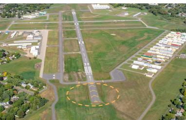
${\it Image showing an example of a Blast Pad at Crystal Airport (MIC)}$
